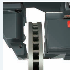
Simultaneous dual-face turning of disk brake
