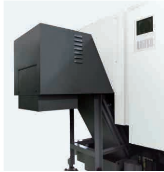
Rear discharge chip conveyor
