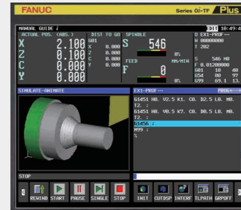
Check cutting result using cutting simulation
