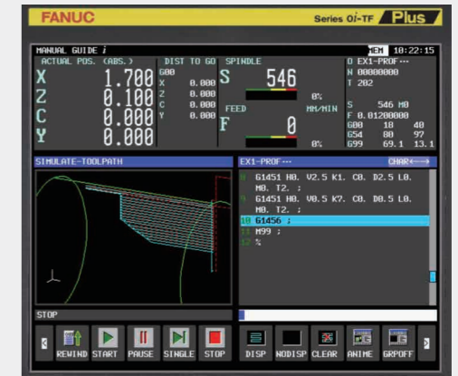
Check cutting path using cutting simulation
