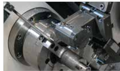
Chuck Air Blow (Upper Chuck)
