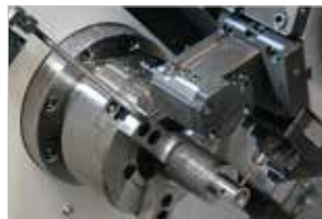
Chuck Air Blow (Upper Chuck)
