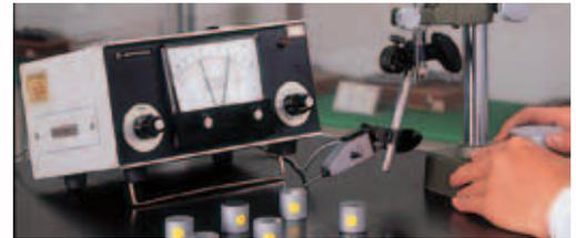
Parallelism of upper and lower sides of the workpiece within 0.002mm (0.0001")
