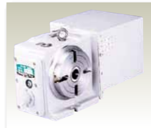
CNC CONTROLLED HORIZONTAL INDEXER (This indexer,driven by AC servo motor and cooperated with CNC controller.) • B45-0802 Resolution: 0.001°/STEP Max.rpm: 33.3rpm The tolerance of positioning is within: 0°0'5"
