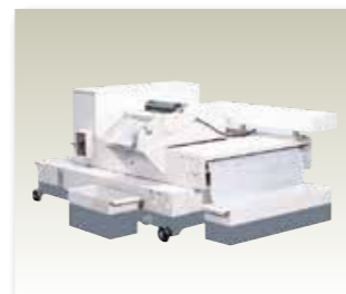
COOLANT SYSTEM WITH AUTO PAPER FEEDING DEVICE&MAGNETIC SEPARATOR (With 1 Roll of Paper) B17-0802(818CNC) Volume: 250L Coolant Capacity: 1/4HPx2 Pump: 80L/min Space: 1600x1100mm (63"x43") Height: 750mm (29 1/2") B17-0806(818CNC) Medium pressure pump:2.3kg/cm 2 Coolant Capacity: 66L/min B17-0807(818CNC) Extra high pressure pump:4.5kg/cm 2 Coolant Capacity: 66L/min B17-1203(C1224CNC) Volume: 500L Extra high pressure pump:4.5kg/cm 2 Coolant Capacity: 66L/min
