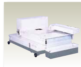
COOLANT SYSTEM WITH AUTO PAPER FEEDING DEVICE (With 1 Roll of Paper) B17-0801(818CNC) Volume: 250L Coolant Capacity: 1/4HPx2 Pump: 80L/min Space: 1600x1100mm (63"x43") Height: 750mm (29 1/2") B17-0803(818CNC) Medium pressure pump:2.3kg/cm 2 Coolant Capacity: 66L/min B17-0804(818CNC) Extra high pressure pump:4.5kg/cm 2 Coolant Capacity: 66L/min B17-1202(C1224CNC) Volume: 500L Extra high pressure pump:4.5kg/cm 2 Coolant Capacity: 66L/min
