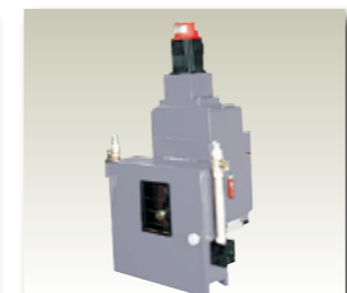
WHEELHEAD MOUNTED AUTOMATIC ROTARY DIAMOND DRESSER WITH AUTO WHEEL DRESSING COMPENSATION(Diamond roller is not included) • B13-0804(818CNC) Motor: 1/4HP Speed: 1750rpm(60HZ) 1450rpm(50HZ) Roller Dia:Max.100mm (3 7/8") Roller Dia:Min.90mm (3 1/8") Clamping width: Max.55mm (2 1/8") Dia of shaft: 35mm (1 3/8") • B13-1204(DIA-3)(C1224CNC) Motor: 2HP Speed: 1750rpm(60HZ) 1450rpm(50HZ) Roller Dia:Max.140mm Spindle Speed: 930rpm(60Hz) 775rpm(50Hz) Dia of shaft: 45mm (1 4/5")
