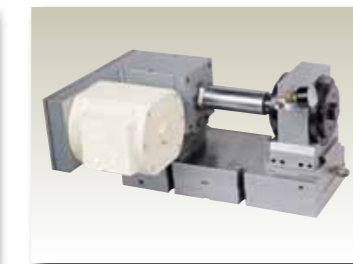
B13-1202 (C1224CNC) Motor:1/4HP Speed:1750rpm(60HZ)/1450rpm(50HZ) Roller Dia: Max.140mm (5 1/2") Roller Dia: Min.90mm (3 1/2") Clamping width:Max. 127mm (5") Dia of shaft: 45mm (1 4/5") B13-1203 Motor:1kw AC SERVO Speed:2000rpm Roller Dia: Max.140mm (5 1/2") Roller Dia: Min.90mm (3 1/2") Clamping width:Max. 200mm (8") Dia of shaft: 45mm (1 4/5")/52mm (2")
