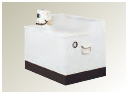
COOLANT SYSTEM WITH DOUBLE FILTER B17-0901X Volume : 95L Pump : 1/8HP Coolant Capacity : 20L/min. Space : 660 x 480mm (26" x 19" ) Height : 610mm (24" )
