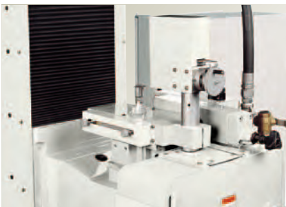
OVER-THE-WHEEL AUTO. STRAIGHT LINE DRESSING & COMPENSATION DEVICE B13-0415X (12 SERIES ) B13-0416X (16 SERIES ) dressing width:70mm(2.75")
