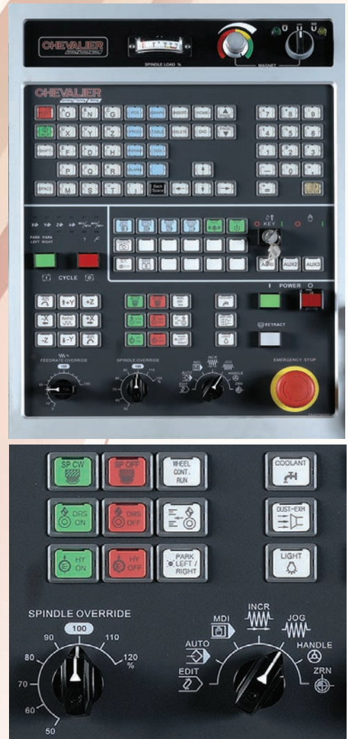
A light has been added to ensure ease of spindle speed monitoring at 100% spindle override position.
